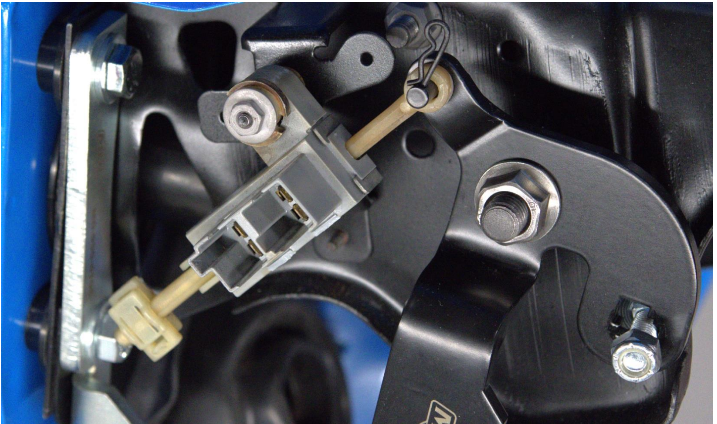
MDL Clutch pedal with carriage bolt/nut, and neutral start switch.
